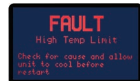
High Temp Limit Fault Screen.
