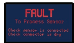
Sensor Probe Fault Screen.
